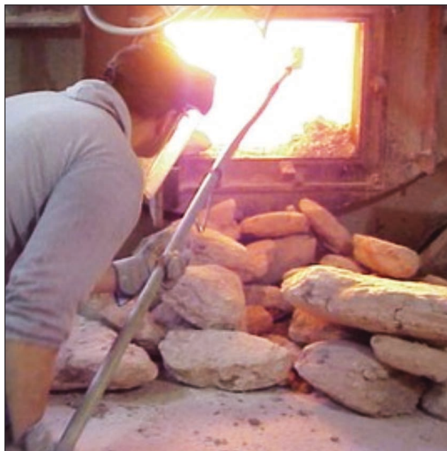
15. Large slabs of fallen ring deposits removed from a lime kiln.
