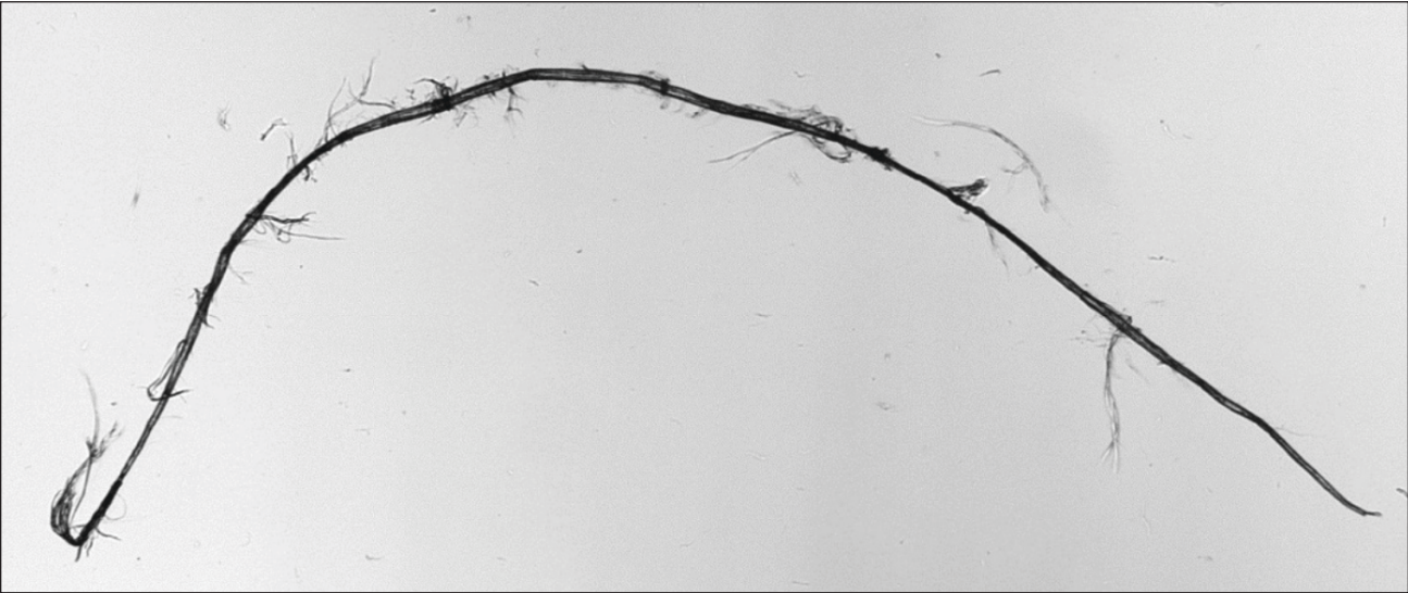
2. Image of a pulp fiber showing external fibrillation.
