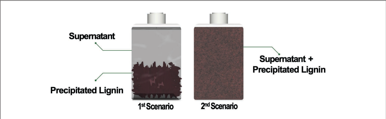
2. Illustrated schematic of two analyzed scenarios of acidulated black liquor (ABL).
