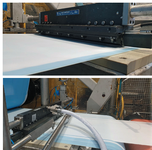
Foam applicator above the vacuum unit in the forming section of the pilot machine. A 100 percent viscose fiber base was used, and latex was applied by foam on top of the wet web.
