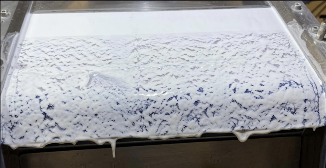
9. Layer separation in wet coating on a curtain coater.
