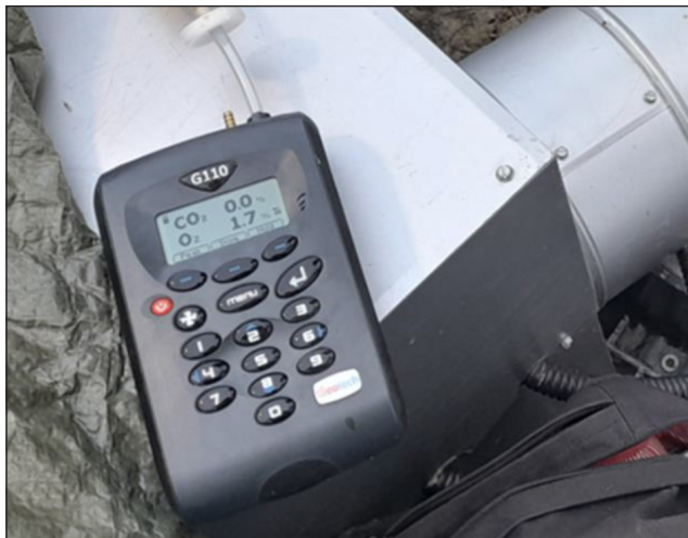
4. The oxygen content of the residual gas in the top of reactor 2 was nearly zero.
