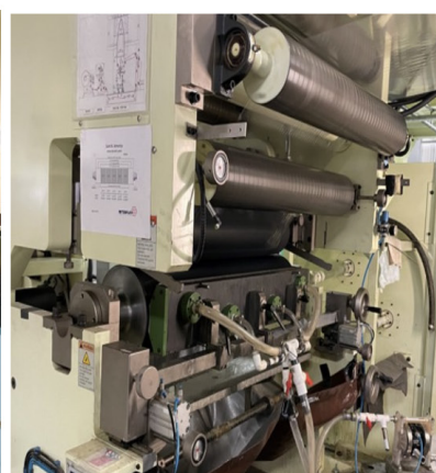
Step 3: Extrusion coating with priming
