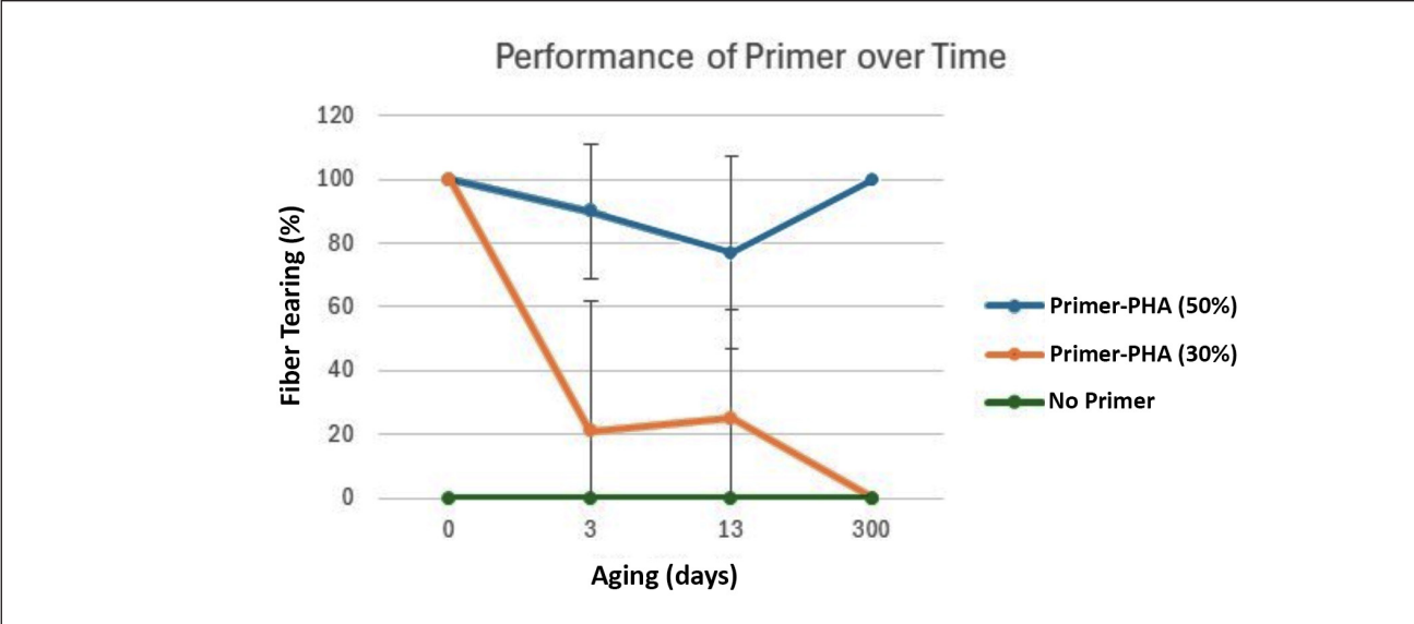
7. The use of primer to avert the aging effect of PHA adhesion. The values shown are the average of all coat weights.
