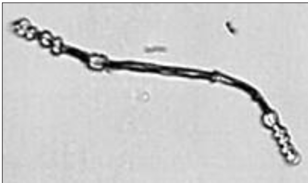
2. Fiber showing localized swelling totalling 36.4% of total length [7].
