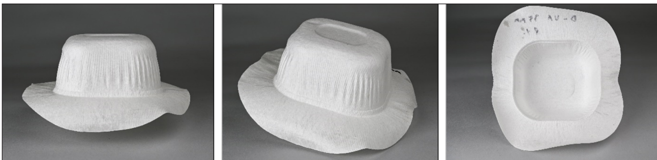
7. Maximum forming depth (35 mm) was prepared using sliding blank forming with the MiniMould tool.
