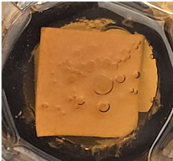
A-9. Photograph showing the gas production under the Kapton foil in the gas detection setup, illustrated in Fig. A-9 with paper I3 after 2 h of irradiation. The first alterations are visible after about 1 to 2 min in radiographs of the scan.
