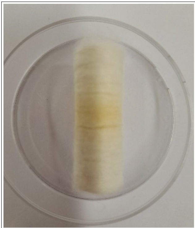
5. A tampon shaped cellulose sample was irradiated in Unitom HR \mu CT at a voltage of 40 kV and a current of 100 \mu A at a SOD of 8.69 mm to sample center (1.69 mm to the sample surface) and for a duration of 16 h and 29 min. The total dose was calculated to 4.35 MGy using Appendix Table A-III.
