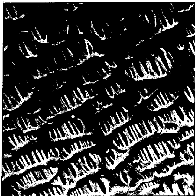
5. Celgard® membrane (7000X magnification) (4)
