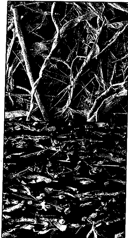
2. Surface (top) and cross section (bottom) of a wet-laid automotive filter paper with microscopic fibers
