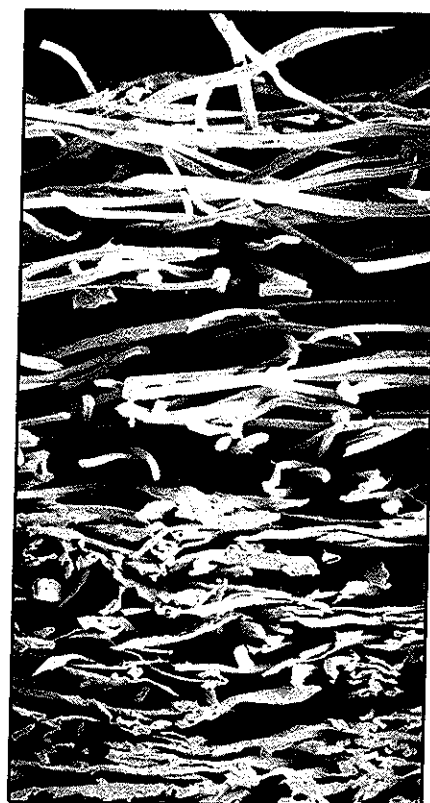
3. Cross section of a gradient-density, automotive, nonwoven filter material
