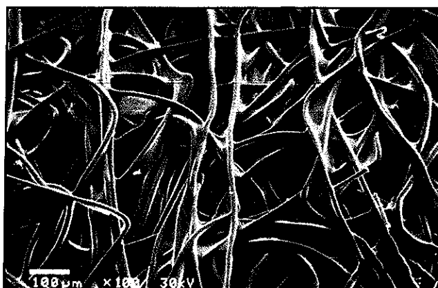
4. Saturation-bonded surface (100x)
