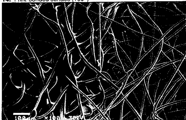
14. Print-bonded surface (100x)
