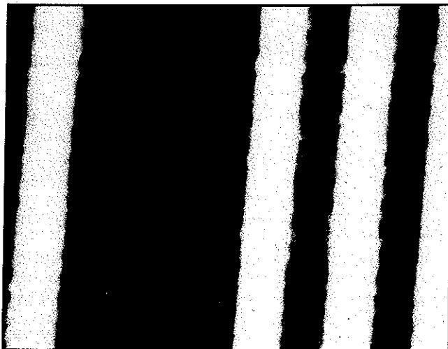
Direct thermal (left) and thermal transfer nonimpact-printed bar codes are magnified 25X.
