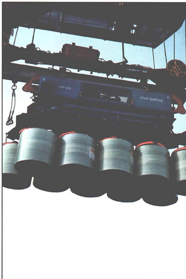
8. Top vacuum loading of ships with Holmens Bruk rolls.
