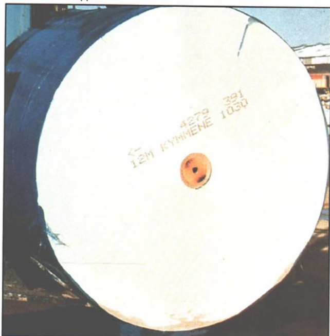
3. Moisture protection test results showed very little damage to the combination wrapped roll.
