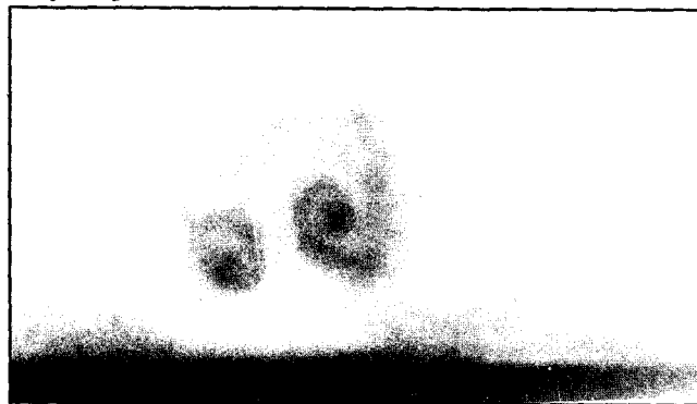
6. Flash X-ray radiographic image of a pair of Taylor-Görtler-like vortices appearing in the vicinity of the downstream secondary roll near the middle of the cavity. Re = 590 , Re^* = 0.35 . The bulk fluid is a typical coating color for rotogravure LWC with 62% solids content. Image magnified to show details.
