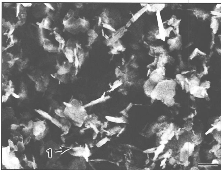
10. Standard nonreactive latex (Latex A) at 5% by wt. in water, etched and then coated with chromium by thermal evaporation. (Bar = 1 \mu\text{m} )
