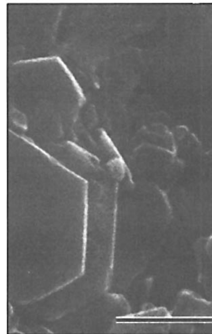
6. Aqueous suspension of 70% by wt. kaolin. Parallel-plate alignments are common. Etched and then sputter-coated with platinum. (Bar = 1 \mu\text{m} )
