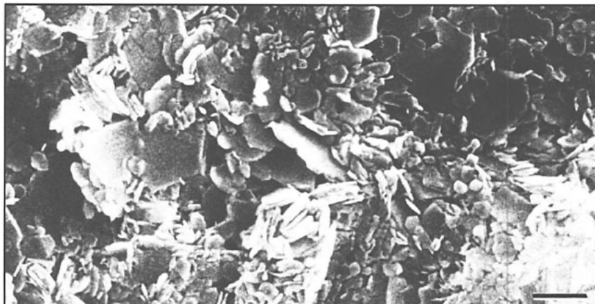
8. Aqueous suspension of 12% by wt. kaolin. Edge-to-edge, edge-to-face, and face-to-face alignments are seen. Platelets are visible partly beneath the ice (7). Etched and then sputter-coated with gold. (Bar = 1 \mu\text{m} ) (7)
