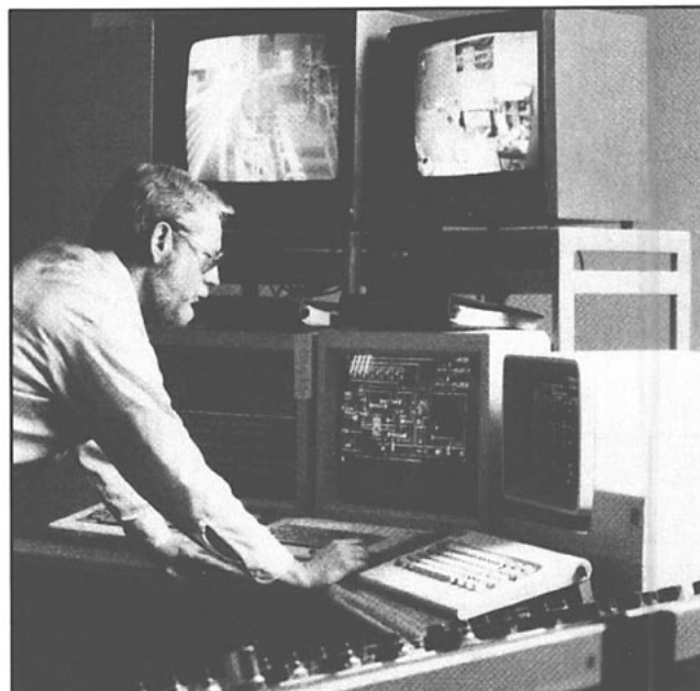
5. An innovative statistical process control system provides necessary graphic data of critical operations at Omya's ultrafine ground calcium carbonate plant in Florence, Vt.
