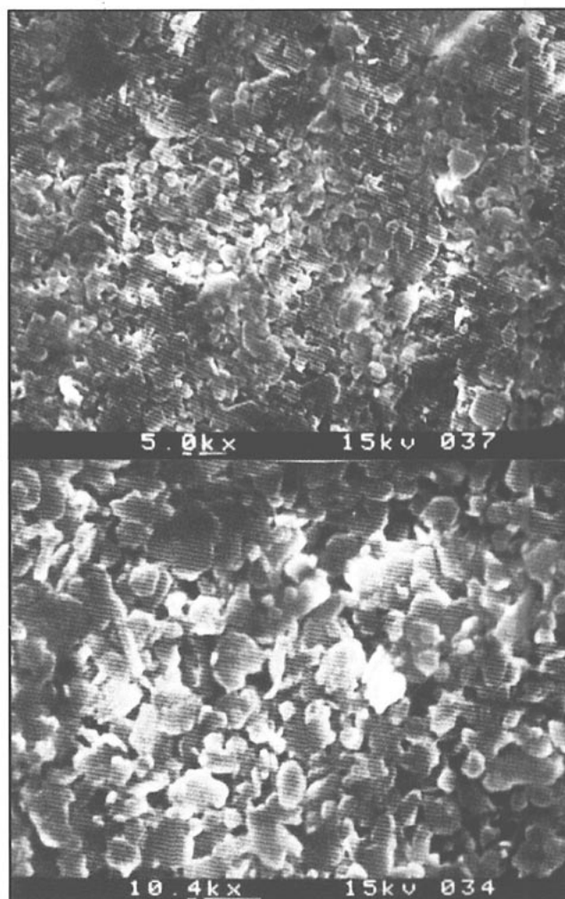
11. SEMs of latex-poor coating surface in valley
