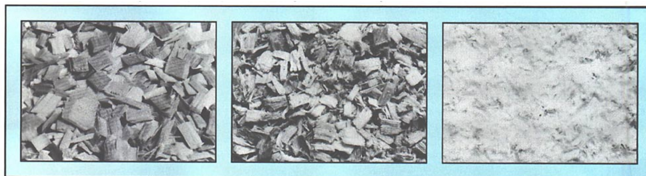
2. The result of proper impregnation: aspen chips before, during, and after two stages of impregnation
