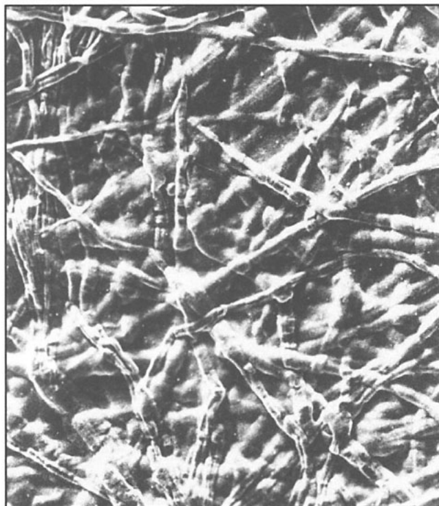
4. Interior surface of casing (100 ×). Viscose binder was applied to exterior surface.
