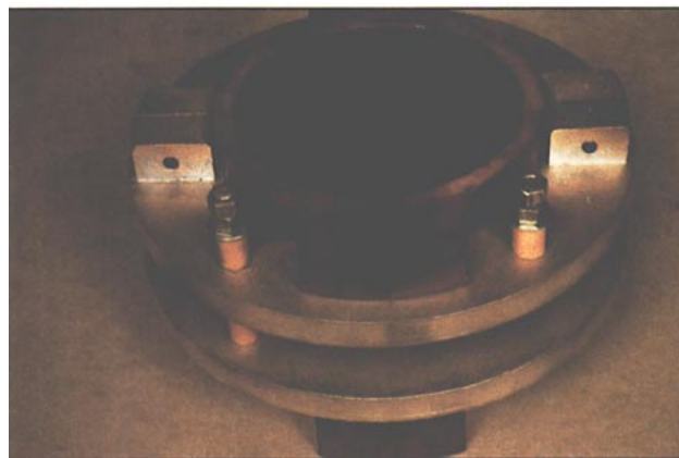
1. Prototype rings showing first design of clamping system used on Textilite hub
