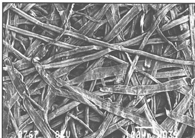
10. Cross-sectional view of the thin-walled juvenile wood fibers in the handsheet of Fig. 8 (marker represents 10 \mu\text{m} )
