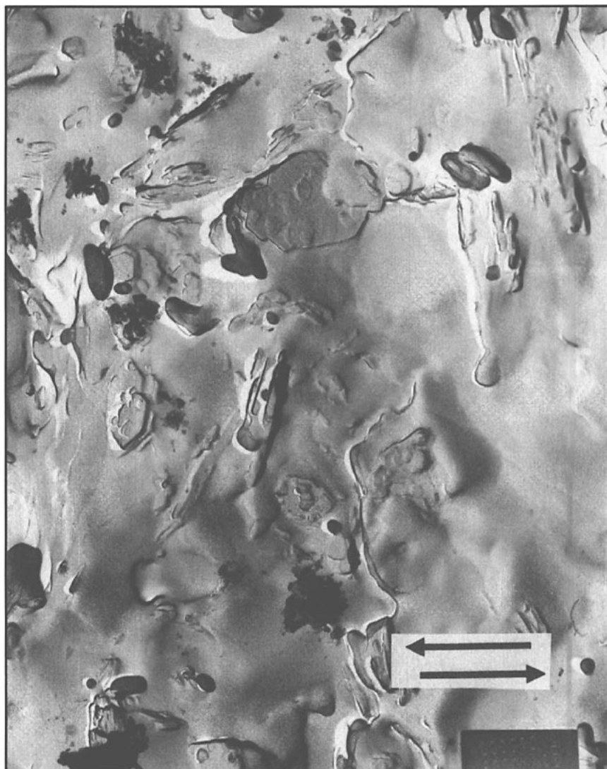
9. Electron micrograph of slam frozen calcined clay—50% solids by weight, 28% solids by volume. Arrows indicate direction of shear. (Magnification 20,000X).
