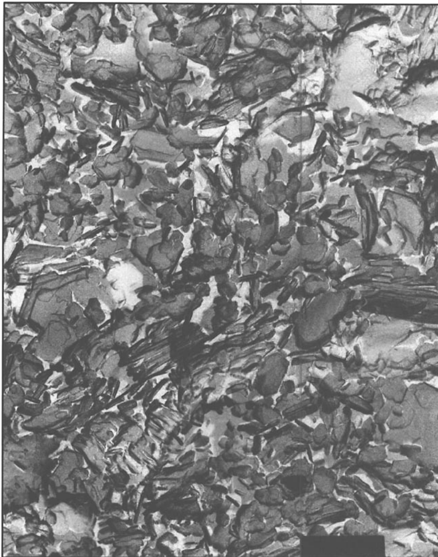
3. Electron micrograph of sample using a static freeze technique. (Magnification 20,000X).
