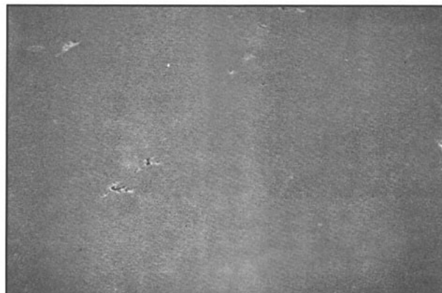
9. Granite; surface finish = 8–25 \mu\text{in. (Ra)} ; magnification \approx 99.5\times .
