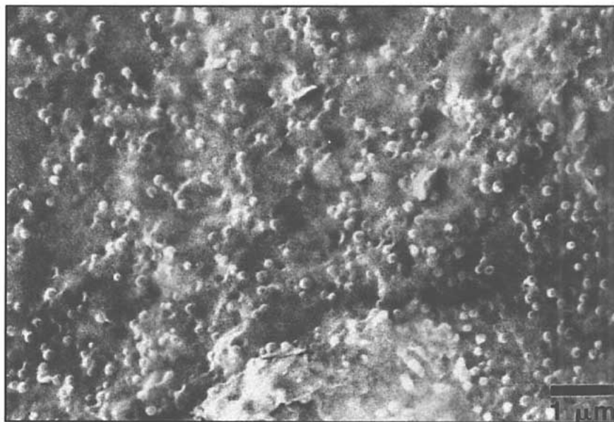
1. Cryo-SEM of fractured, frozen floc of carboxylated polystyrene-butadiene HC latex
