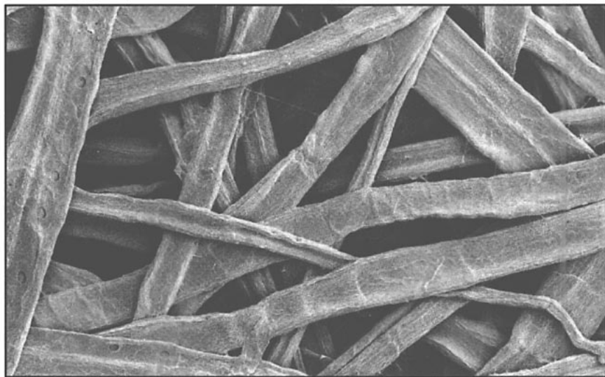
17. Surface of an unbleached kraft pulp handsheet made from mature wood of second-growth lodgepole pine. Fiber coarseness is 281 \mu\text{g}/\text{m} . (The marker is 100 \mu\text{m} in length.)
