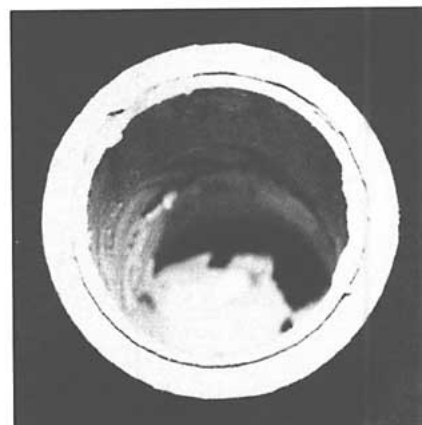
4. Initial failure of a core
