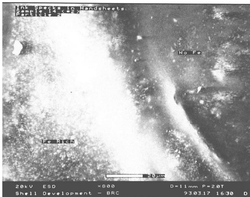
12. ESEM image of a residual MOP ink particle after pilot mill pulping at 160°F
