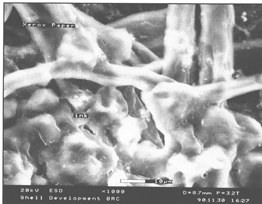
3. Enlargement of Fig. 2. Note the partial fusion of toner particles and their attachment to fibers.
