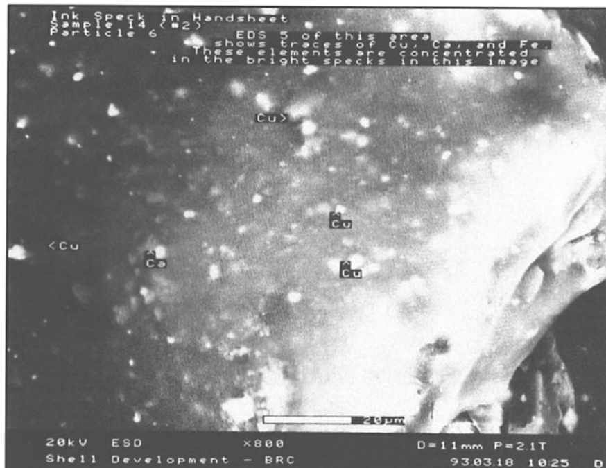
12. ESEM image of a residual MOP ink particle after pilot mill pulping at 160°F
