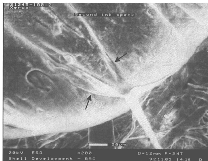
4. ESEM image of a residual photocopier styrene-acrylate toner ink particle after laboratory pulping and flotation at 110°F using SDA-30.
