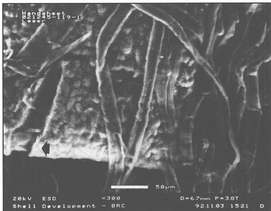
6. ESE micrograph of a residual polyester resin laser ink particle after laboratory repulping and flotation at 200°F using SDA-30.
