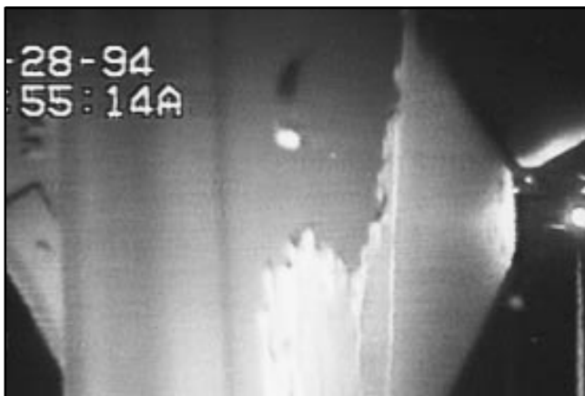
16. Bubble approximately 61 cm (24 in.) from the sheet edge
