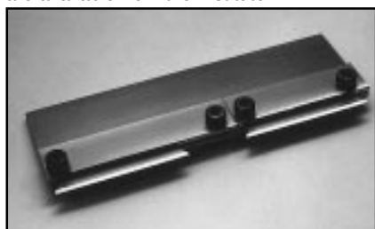
7. The jig for making edge notches in paper specimens. Details of the clamps and the jig are available from the Institute.
