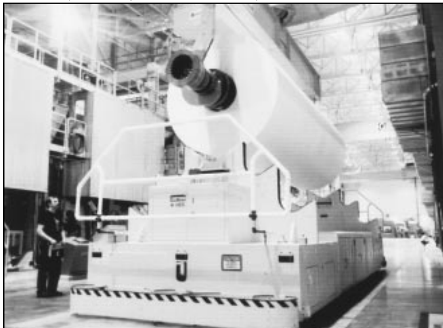
2. Reel and spool handling AGV in the No. 16 facility
