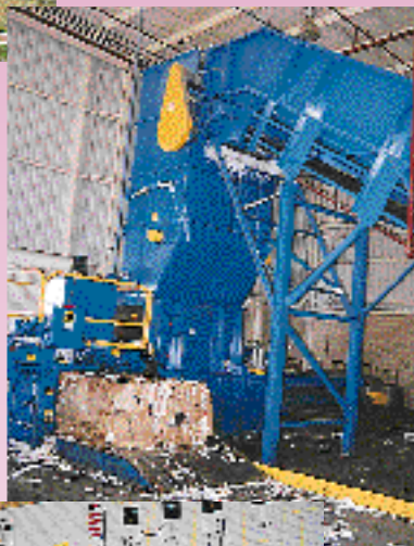
This baler packages tons of sorted recovered papers.
