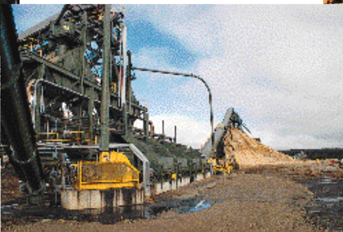
Oversized pieces are removed before the chips are conveyed to the chip pile.
