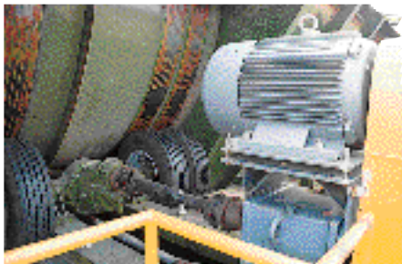
Truck tires and axles transfer the driving force to the drum debarker
