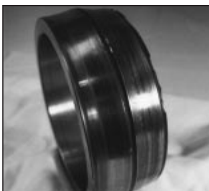
7. Excessive clearance reduction
