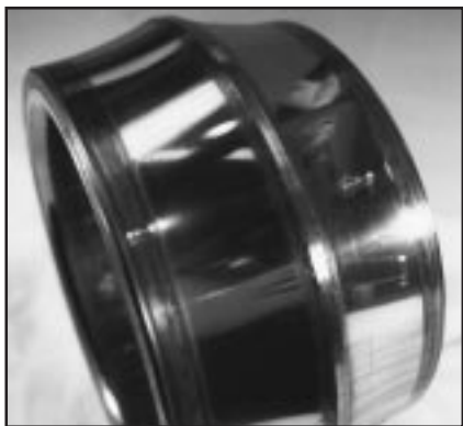
16. Inadequate lubrication or polishing wear
