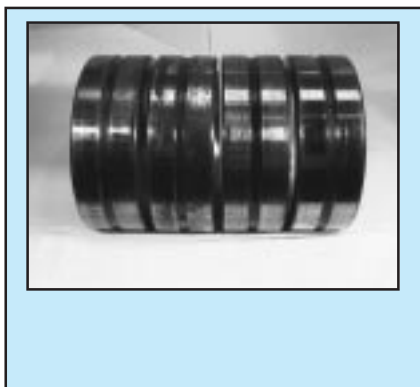
10. Housing fit too loose
