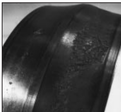
11. Thrust load failure
