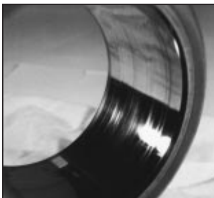
5. Insufficient interference fit on shaft
