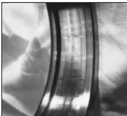
1. Damage caused by false brinell
