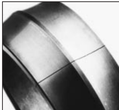
6. Excessive interference fit
