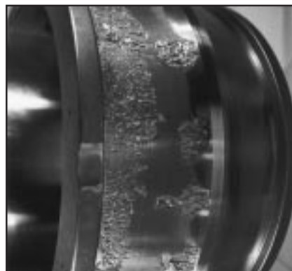
23. Advanced stage of spalling initiated during a nonrotating condition
