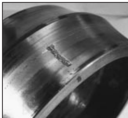
22. Progressed state of spalling initiated by static corrosion
