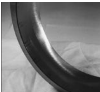
4. Damage caused by inspection
