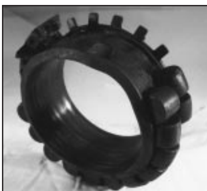
8. Excessive operating temperature
