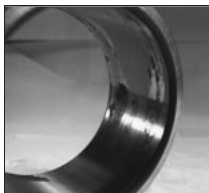
9. Improper fit on shaft
