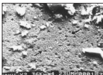
8. Tunnel formation in nodules over galvanized iron, 2360X SEM
