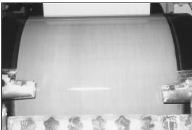
14. Photograph of premetered film on roll at 8 g/m² and 62% solids
