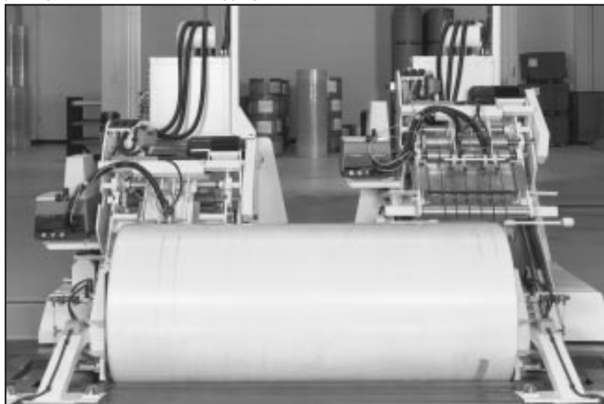
3. A kraft wrapping head (left) and a film wrapping head (right) spirally apply separate layers of pure kraft paper and polyethylene to the roll circumference, producing a fully recyclable package. The same width of wrapping material is used for all roll widths.
