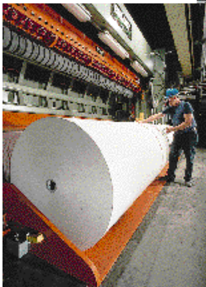
(above) An operator works in front of Fraser's soft-nip calender on PM5
