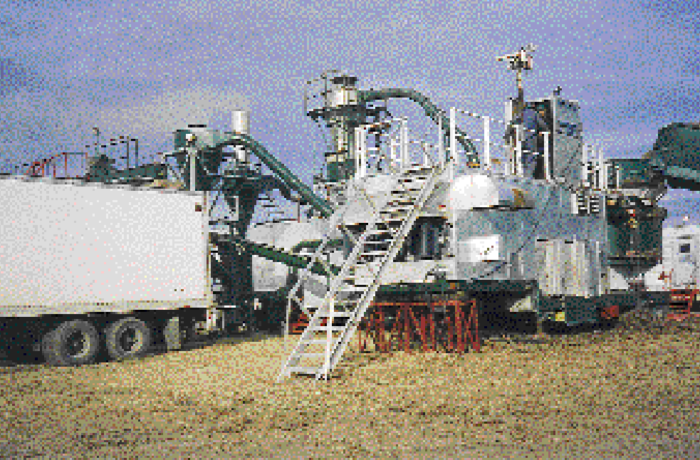
Dust and shive removal section at Treherne, Manitoba
