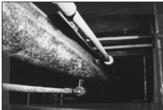
12. Anodic protection with centrally-mounted cathodes
