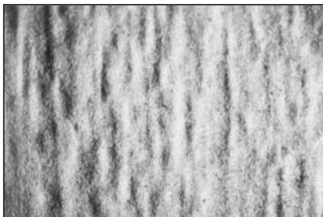
5. Nonuniform thinning in the wash zone of a continuous digester
