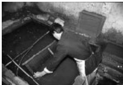
China - Forming mulberry pulp on a bamboo screen held to a wood frame with deckle sticks (Koretsky)
