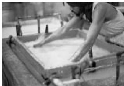
India - Sheet forming using a deckle-box type mould (Koretsky)
