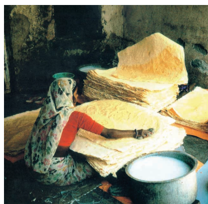
India - Sizing the surface of each sheet with boiled flour paste (Neeta Premchand/"Off the Deckle Edge")
