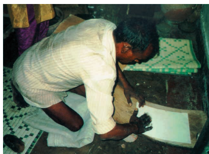
India - Polishing a finished sheet on a concave wooden pillow with an agate embedded in a lump of clay (Neeta Premchand/"Off the Deckle Edge")
