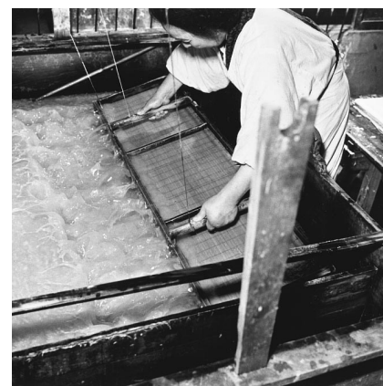
Japan - Dipping the mould into slurry treated with viscous tororo aoi (RCWAMP)
