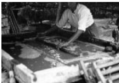
Myanmar - Removing air bubbles from the pulp using a bamboo rod (Koretsky)
