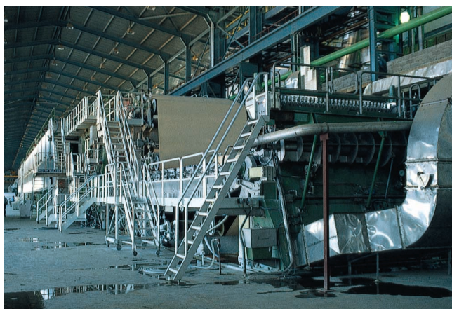
The forming section of the new Voith paper machine
