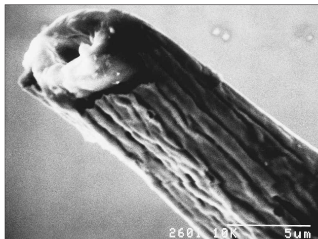
3. A single kenaf fiber cell with a narrow lumen and a thick wall
