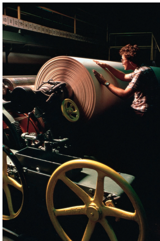
5. Manual inspection of the roll
