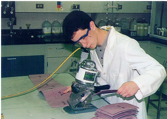
A lab technician prepares the wet press felt for physical testing. (Courtesy of DuBois Paper Technology).
