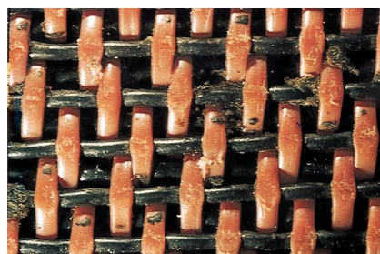
11. New design with hollow weft on a contamination prone position after cleaning
