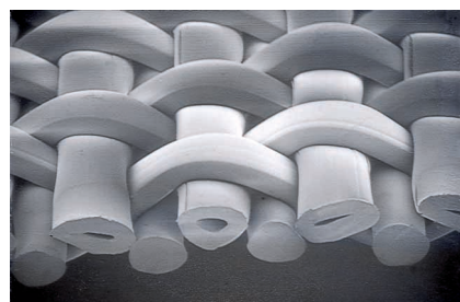
6. Pattern woven with a combination of solid and hollow monofilaments
