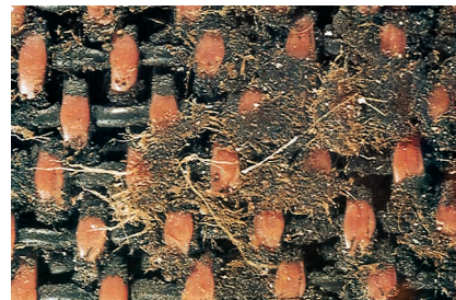
10. New design with hollow weft on a contamination prone position before cleaning
