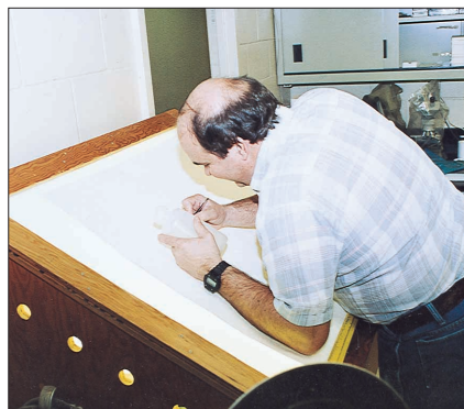
1. Inspection for plastic using the light box technique
