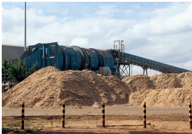
The drum debarker and chip storage
