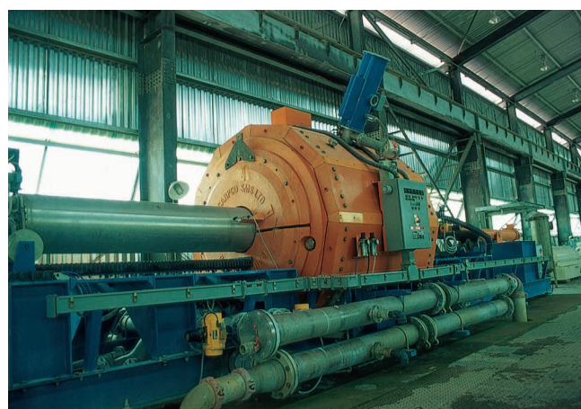
RCC's cryogenic electromagnet removes iron particles from the clay
