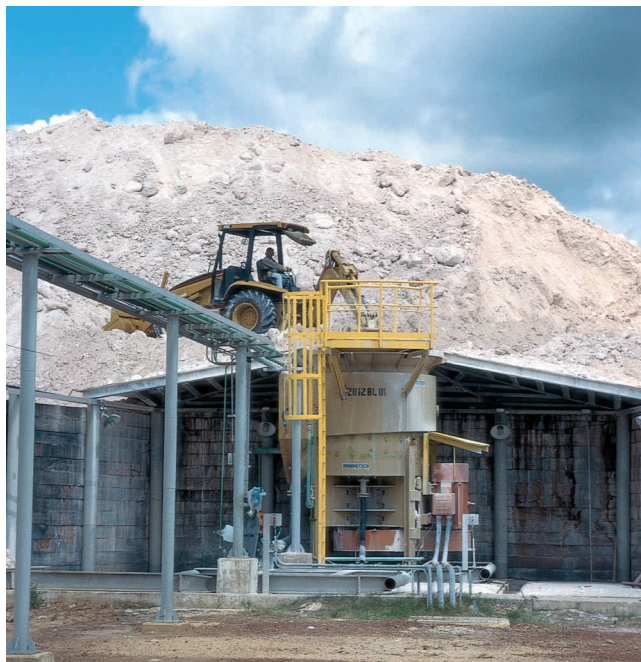
A bulldozer moves raw kaolin from storage to the blunger.
